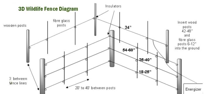
that are energized. The second, outside line of fence has one high-tensile wire that is also energized. The gates of the enclosure should to be energized as well, as they are weak points.
